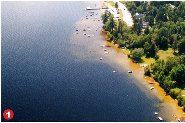
1 THE TOWN DOCK SHORE A significant sedimentary deposit has built up at the mouth of the creek about 100 metres north-west of the town dock. Shallow water extends out about 50 metres from the shore.
